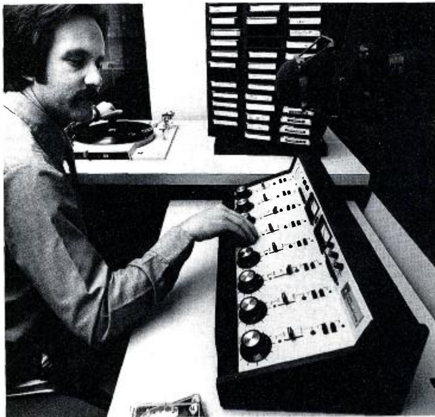
New Cetec Model 2003 8-mixer audio console.
